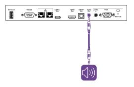
In addition to the Stereo 3.5 mm Out connector, the display provides a Sony/Philips Digital Interface (S/PDIF) Out connector. S/PDIF is a digital audio transmission medium. You need an audio system that has an S/PDIF input to decode this connection to analog. Most external sound bars include an S/PDIF connector.
